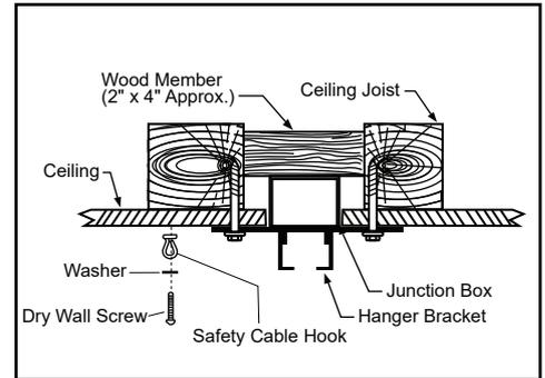
Tighten the hanger bracket to the outlet box with two mounting screws. **(Make sure the outlet box is securely installed so that it will be able to support at least the fan weight.)** Attach the safety cable hook to the ceiling with the dry wall screw and washer, and make sure the safety cable hook is covered by the fan canopy.
