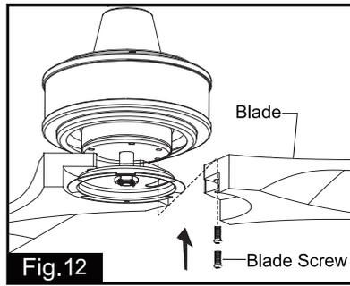
Attach blades to blade brackets by using blade screws. (Do not lock the two blades that are installed first, and lock them together after the third blade is installed.)
