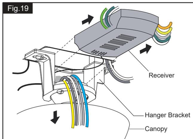
Unscrew the canopy. Remove the wire connectors from the fan to ceiling wire connection. The receiver should be removed from the hanger bracket. (See Fig.19)
