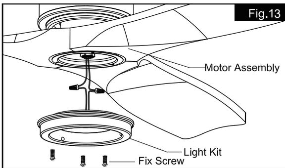
Connect the blue wire from motor to the black wire from light kit by wire connectors. And connect the white wire from motor to the white wire from light kit by wire connectors. Remove three fix screw from bottom of motor assembly (for later use). Secure the light kit to motor assembly with previous three fix screw.
