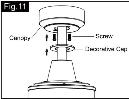
Secure the canopy to hanger bracket with screws. Attach the decorative cap to the canopy and rotate the decorative cap clockwise until it locks in place.
