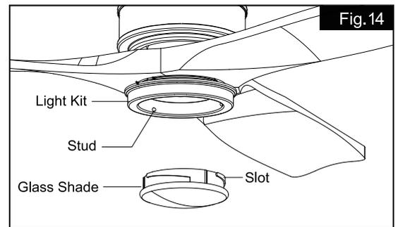
Attach the glass shade to the light kit by aligning studs and slots, and turn it clockwise until it is locked in place.
