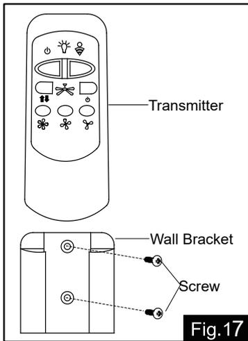
Install the transmitter wall bracket in wall by two screws and hang transmitter in it carefully.
